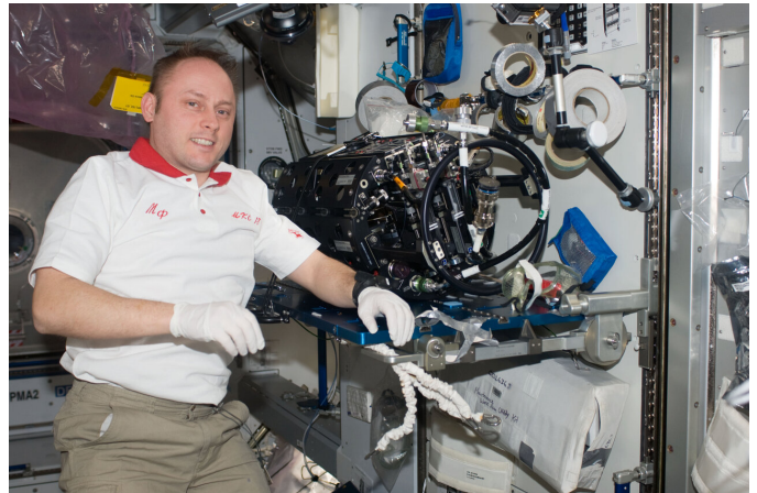
Astronaut Michael Fincke, Expedition 18 commander, works on the Multi-User Droplet Combustion Apparatus (MDCA) Chamber Insert Assembly (CIA) in the Harmony node of the International Space Station. Credit: NASA
