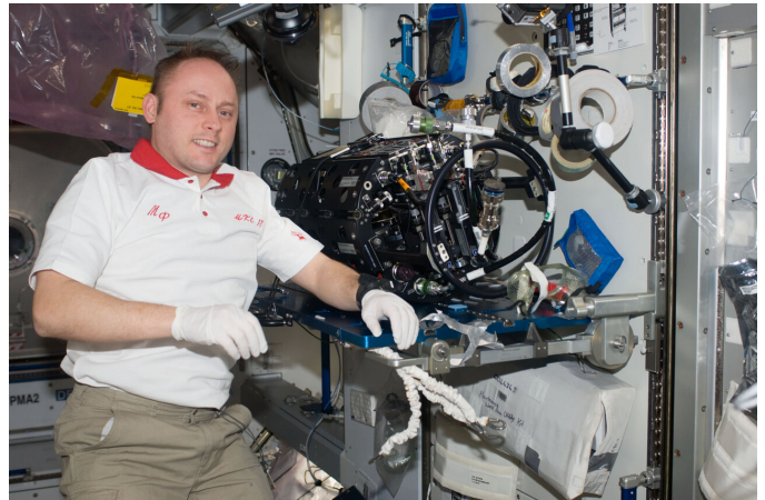
Astronaut Michael Fincke, Expedition 18 commander, works on the Multi-User Droplet Combustion Apparatus (MDCA) Chamber Insert Assembly (CIA) in the Harmony node of the International Space Station. Credit: NASA
