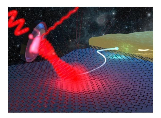
The image depicts a schematic of terahertz (THz) heterodyne detection with graphene. In this, two THz waves (red) are coupled into graphene, where they are combined or mixed. One of the waves is a high intensity signal generated by a local THz light source (i.e. a local oscillator), at a known THz frequency. The other signal is a faint THz wave that mimics the waves coming from space. Credit: Photographer / Source Hans He
