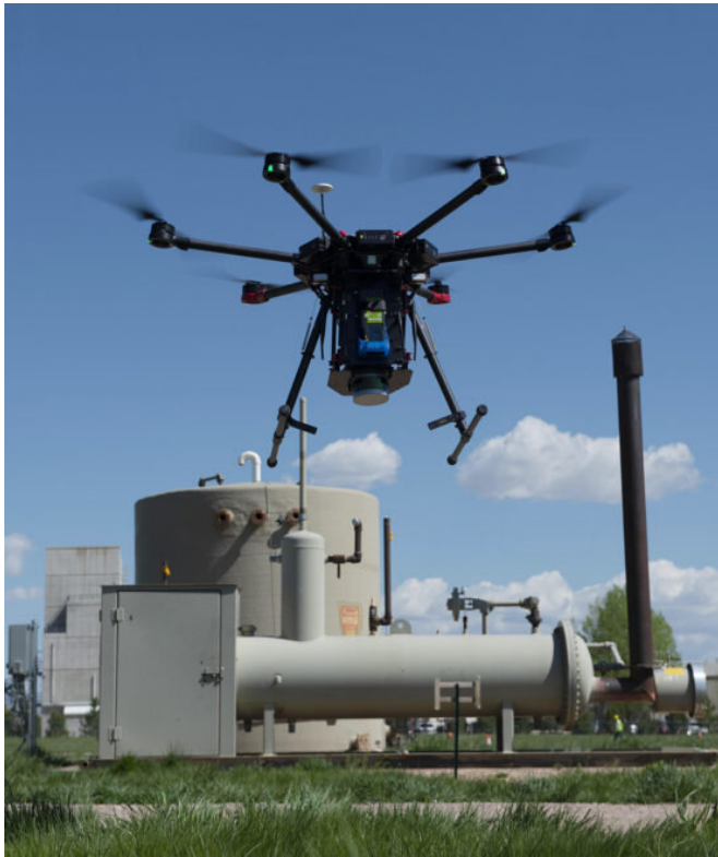
A drone sniffs for methane leaks in the Mobile Monitoring Challenge at the test site in Colorado. Credit: Sean Boggs/Environmental Defense Fund
