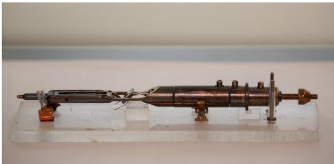
MIT Professor Frances Ross has designed several custom sample holders for examining nanoscale materials in gases and liquid media in the electron microscope. For liquid environments, thin windows of silicon nitride surround the liquid but allow the electron beam to pass through. For gas environments, the sample holder (shown here) must heat and tilt the sample without compromising its cleanliness. Credit: Denis Paiste/Materials Research Laboratory
