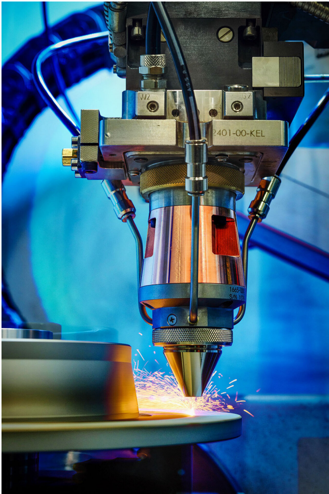
Coating a brake disc with the EHLA process. Credit: Fraunhofer ILT, Aachen, Germany / Volker Lannert
