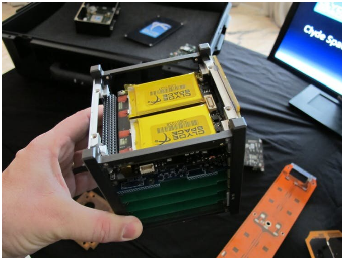
1U CubeSat structure. Credit: wikipedia, CC BY-SA
