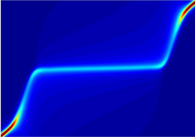
A plot of the electron spectral function for the important current-carrying electrons in energy-momentum space. Credit: Patel & Sachdev.
