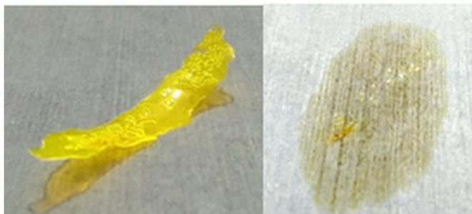
A polymer (left) depolymerizes and disappears after being exposed to sunlight for 10 min (right). Credit: Paul Kohl
