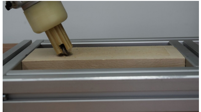
A robot that used force-control technology developed by Ludovic Righetti and Johannes Pflöging tested the adhesive by scraping a block of wood 170 times. Credit: NYU Tandon, Johannes Pflöging
