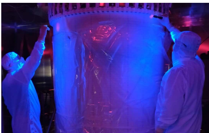
The detector is inspected under UV light. Credit: Nicolas Angelides
