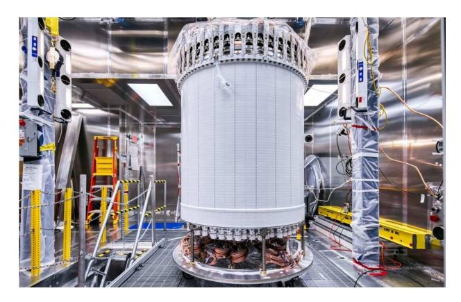
The recently assembled LUX-ZEPLIN xenon detector in the Surface Assembly Lab cleanroom at Sanford Underground Research Facility on 26 July 2019. Credit: Matt Kapust.
