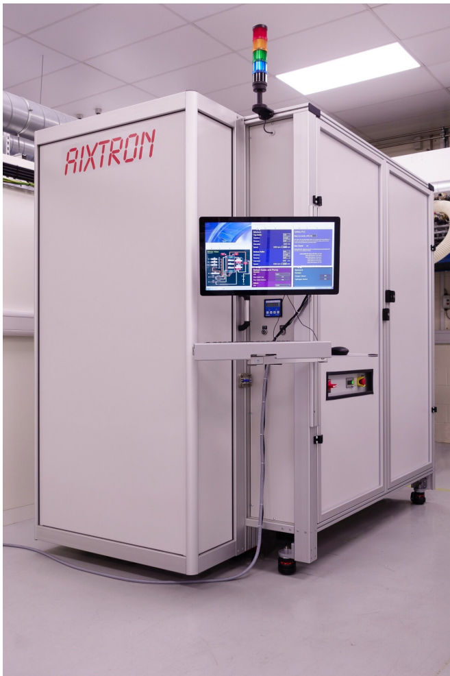
AIXTRON's new 'Neutron' roll to roll system for the production of graphene. Credit: AIXTRON / Graphene Flagship
