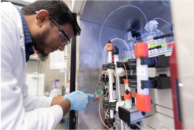
Umar Hameed performs size-exclusion chromatography, an important step in the purification of proteins. Credit: KAUST
