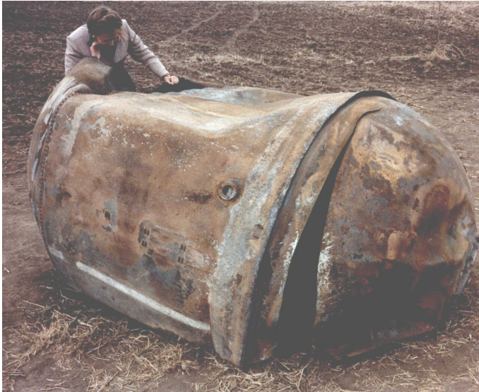
The main propellant tank of the second stage of a Delta 2 rocket landed near Georgetown, Texas, USA, on 22 January 1997. This tank of about 250 kg is primarily a stainless steel structure and survived reentry relatively intact. Credit: NASA
