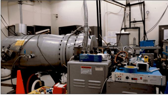
A particle accelerator at the Radiation Effects Facility hurls high-energy particles at instruments, mimicking the solar wind or galactic cosmic rays. Credit: NASA's Goddard Space Flight Center/Genna Duberstein
