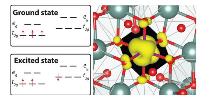
QMCPack can be used to calculate the ground and excited state energies of localized defects in insulators and semiconductors—for example, in manganese (Mn)<sup>4+</sup>-doped phosphors, which are promising materials for improving the color quality and luminosity of white-light-emitting diodes. Credit: Brookhaven National Laboratory
