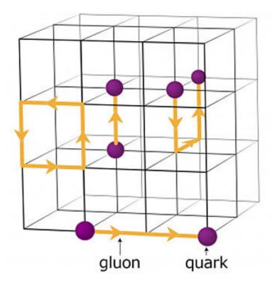
A schematic of the lattice for quantum chromodynamics calculations. The intersection points on the grid represent quark values, while the lines between them represent gluon values. Credit: Brookhaven National Laboratory
