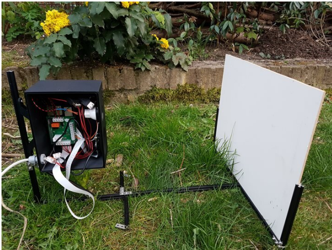
A prototype of the camera trap. Credit: Radboud University
