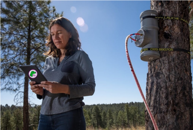
Mariah Carbone uses the Flux Puppy to measure carbon dioxide. Credit: Northern Arizona University
