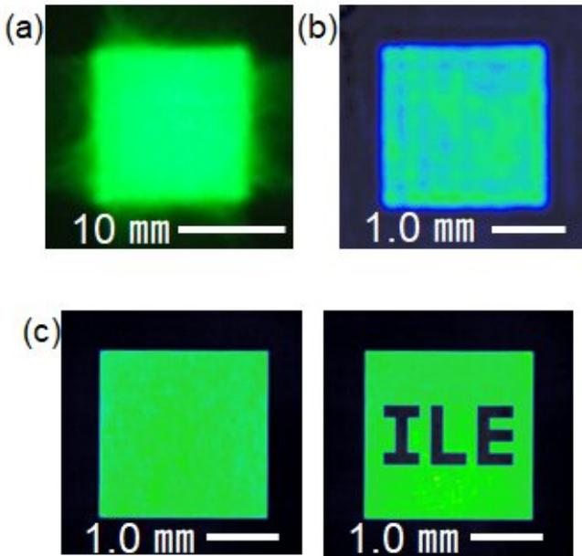
Figure 1. Square flattop beam profiles made by: (a) Diffractive Optical Element (DOE), (b) vertical phase grating (conventional method), (c) virtual diagonal phase grating (new method). Credit: © 2019 Nakata Y. et al., *Scientific Reports*.
