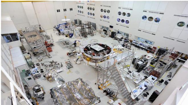
In the center of this image is the Mars 2020 spacecraft stack attached to the Spacecraft Assembly Rotation Fixture (SCARF) in the High Bay 1 clean room in JPL's Spacecraft Assembly Facility. Credit: NASA/JPL-Caltech
