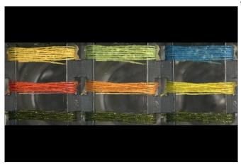
Sensing threads prepared with bromothymol blue (top thread), methyl red (middle thread) and MnTPP (bottom thread) are exposed to ammonia at 0 ppm (left panel) 50 ppm (middle panel) and 1000 ppm (right panel). Credit: Rachel Owyeung, Tufts University, Nano Lab
