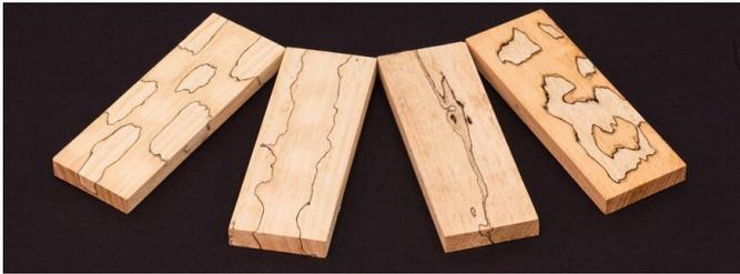
Marbled wood from the lab: Depending on the kind of fungi used, the course of the pattern in the wood can be controlled. Credit: Empa
