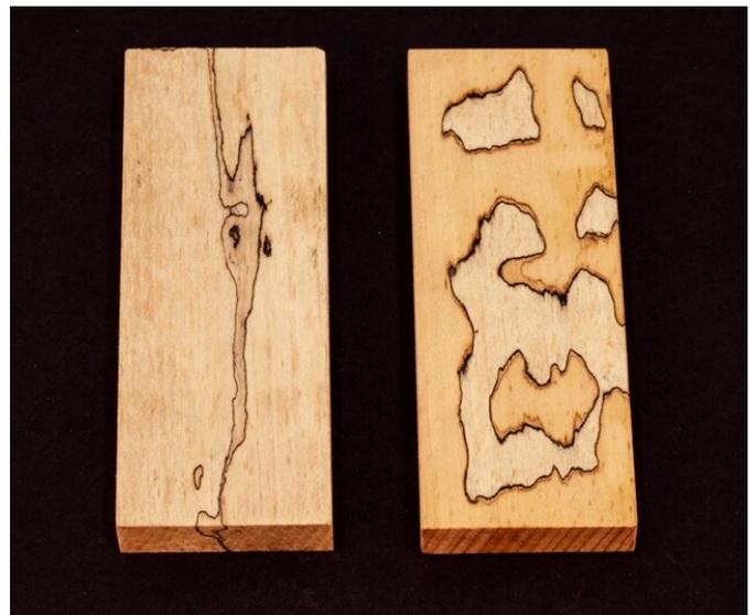
Marbled wood from the lab: Depending on the kind of fungi used, the course of the pattern in the wood can be controlled. Credit: Empa
