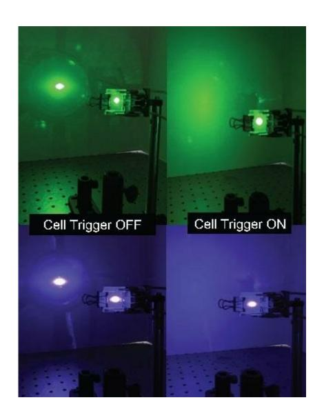
Liquid crystals sandwiched between two1-inch squares of glass scatter green and blue light on a wall when the cells are triggered by laser illumination (right panels). Credit: Daniel Maurer
