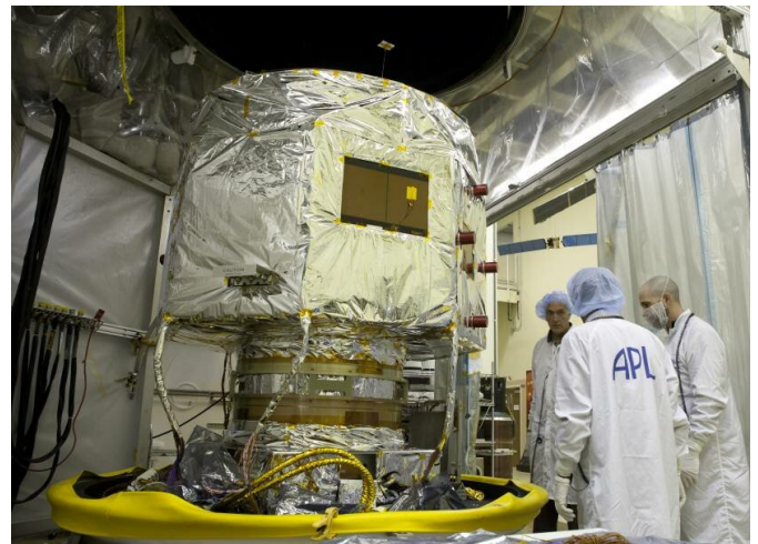
In late 2010, engineers at the Johns Hopkins Applied Physics Laboratory prepare to place Van Allen Probes spacecraft "B" in a thermal-vacuum chamber, where the propulsion system would be tested to ensure it could stand up to the range of hot, cold, and airless conditions of outer space. Credit: NASA / JHU APL / Ed Whitman
