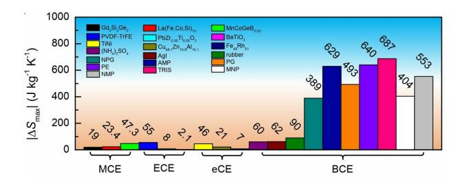
MCE: magnetoclaoric effect; ECE: electrocaloric effect; eCE: elastocaloric effect; BCE: barocaloric effect. The plastic crystals identified in the present work are neopentylglycol (NPG), pentaglycerin (PG), pentaerythritol (PE), 2-Amino-2-methyl-1,3-propanediol (AMP), tris (hydroxymethyl) aminomethane (TRIS), 2-Methyl-2-nitro-1-propanol (MNP), 2-Nitro-2-methyl-1,3-propanediol (NMP). Credit: Huang Chengyu
