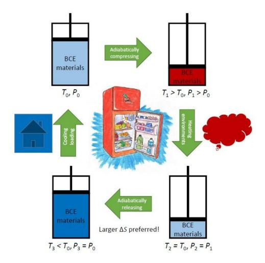
Schematic diagram of the refrigeration cycle based on barocaloric effects. Credit: Huang Chengyu
