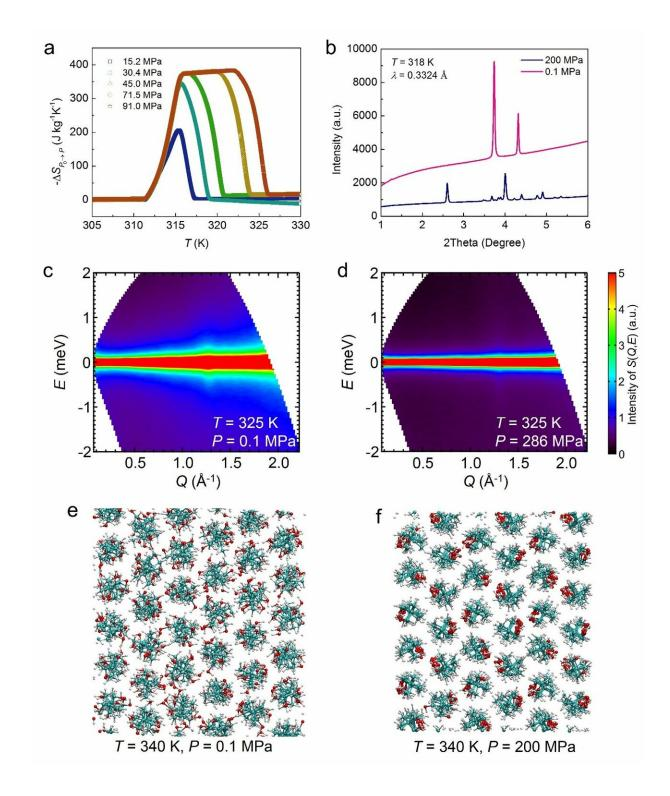
(a). Pressure-induced entropy changes as a function of temperature under varying pressures. (b). X-ray diffraction patterns, showing a pressure-induced phase transition. (c,d). Neutron scattering spectra, displaying that the pressure
