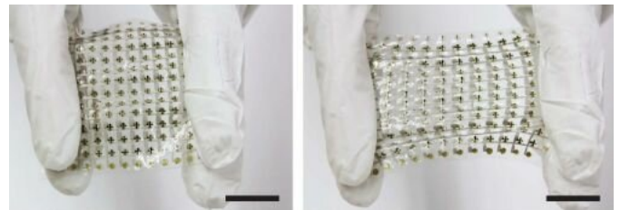
Image 1: A wide range of stretchable electronic devices are being investigated, including this thin-film transistor matrix, showed relaxed (L) and stretched to about 60% (R). The transistor parameters remain almost unchanged upon stretching up to 140%. Credit: Matsuhisa, N. et al. Nature Communications. 25 July 2015/Creative Commons
