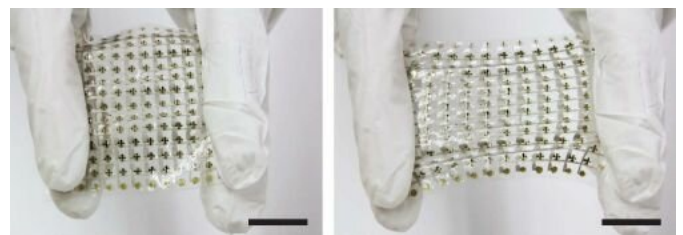
Image 1: A wide range of stretchable electronic devices are being investigated, including this thin-film transistor matrix, showed relaxed (L) and stretched to about 60% (R). The transistor parameters remain almost unchanged upon stretching up to 140%. Credit: Matsuhisa, N. et al. Nature Communications. 25 July 2015/Creative Commons
