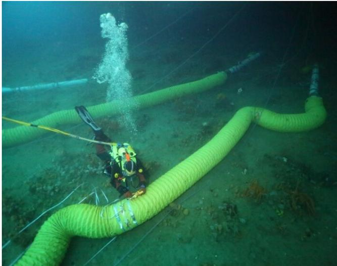
These large tubes are part of the antFOCE system. Chemical reactions occur more slowly in the frigid waters of the Antarctic, so these 30-meter-long tubes allow time for CO<sub>2</sub>-saturated seawater to become more acidified before it flows into the antFOCE experimental chamber. Credit: Glenn Johnstone
