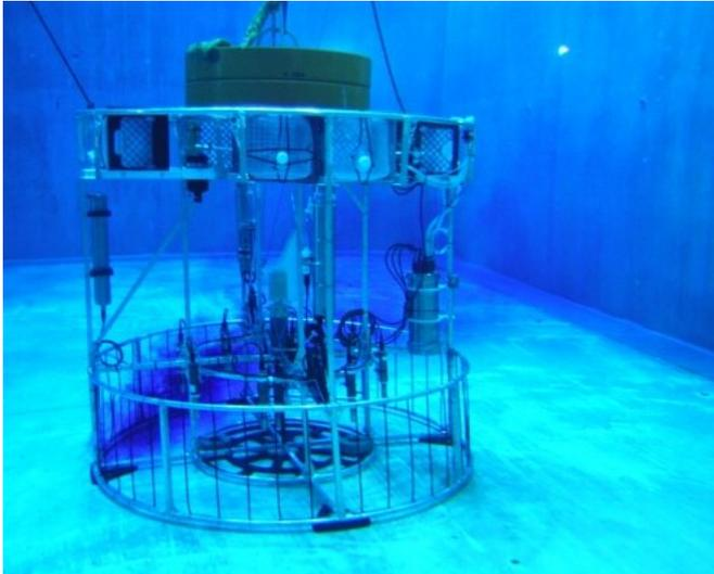
Modeled after similar systems on land, this first-generation FOCE system in MBARI's test tank used a circular frame to release carbon dioxide-enriched seawater into a central chamber. Credit: MBARI
