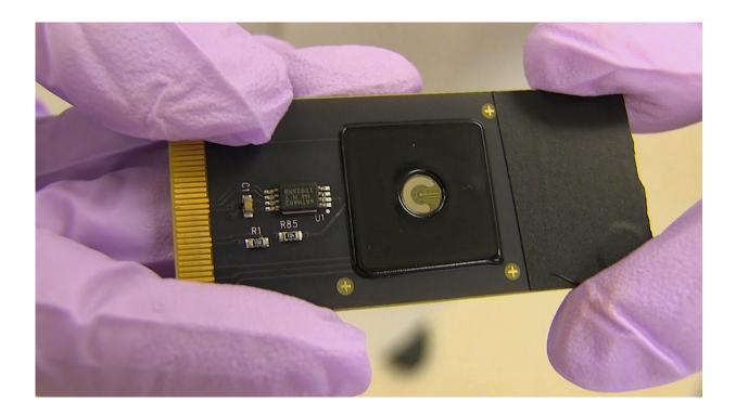
To harness CRISPR's gene-targeting ability, the researchers took a deactivated Cas9 protein -- a variant of Cas9 that can find a specific location on DNA, but doesn't cut it -- and tethered it to transistors made of graphene. When the CRISPR complex finds the spot on the DNA that it is targeting, it binds to it and triggers a change in the electrical conductance of the graphene, which, in turn, changes the electrical characteristics of the transistor. Credit: Keck Graduate Institute
