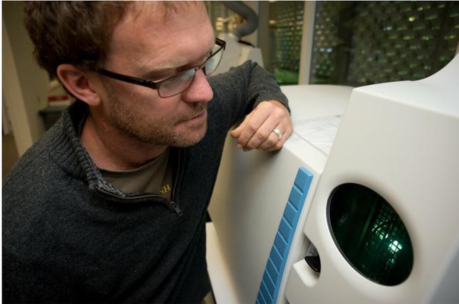
Oregon State University geologist Adam Kent uses a laser ablation machine to measure chemical compositions in volcanic rock. Credit: Jeff Basinger
