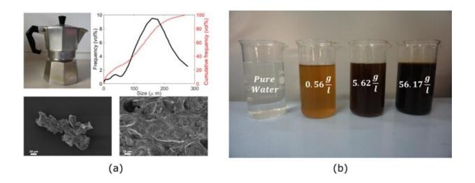
Synthesis of coffee-based colloids. (a) Coffee pot moka used for coffee preparation (top-left); size distributions of the suspended coffee particles (top-right); Scanning Electron Microscopy (SEM) images of the coffee particles (bottom). (b) Colloids with different G30 concentration (from right to left): pure G30 fluid (56.17 g/l of suspended particles); G30w10 fluid (10% dilution); G30w1 fluid (1% dilution in water); pure water. Credit: *Scientific Reports*, doi: 10.1038/s41598-019-39032-5
