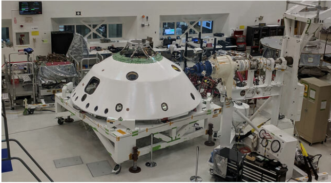
With the backshell that will help protect the Mars 2020 rover during its descent into the Martian atmosphere visible in the foreground, a technician on the project monitors the progress of Systems Test 1. Credit: NASA/JPL-Caltech
