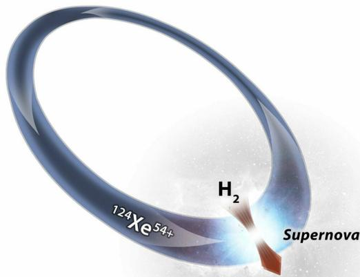
For the first time, the fusion of hydrogen and xenon was able to be investigated at the same temperatures as occur in stellar explosions using an ion storage ring. Credit: Mario Weigand
