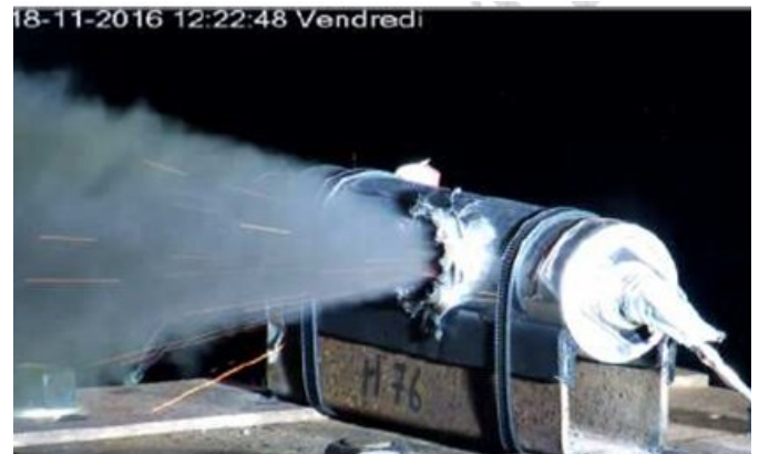
To simulate a micrometeoroid impact an 8 mm bullet was fired into a space battery cell to simulate a micrometeoroid impact. Credit: ESA/Airbus
