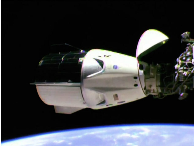
The SpaceX Crew Dragon is docked to the International Space Station. Credit: NASA TV
