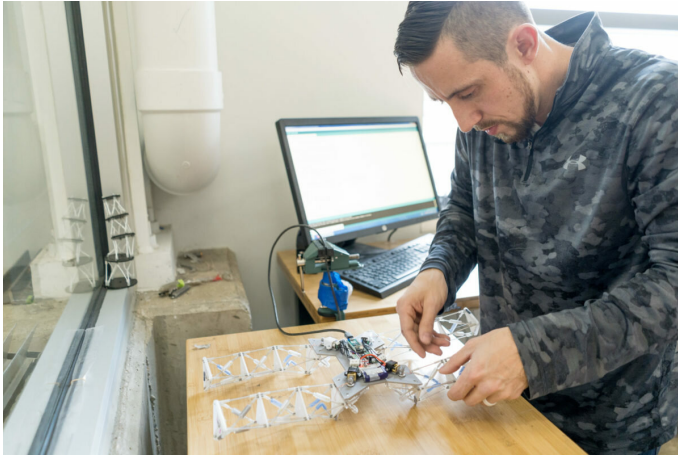
Undergraduate researcher Brandon Tighe with a reconfigurable robot designed to use its legs to both walk and grasp. Credit: Colorado State University
