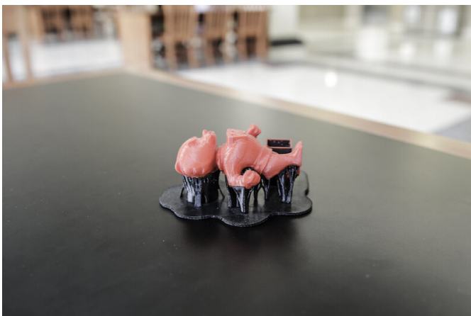
Qian's new method reduces the amount of support material (black plastic) needed to allow the red material (Bucky) to be 3D-printed. Credit: Sarah Page
