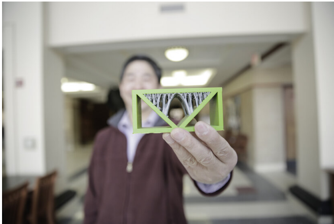
Xiaoping Qian holding a 3-D-printed beam. The silver parts are the optimized support structure for the beam. Credit: Sarah Page
