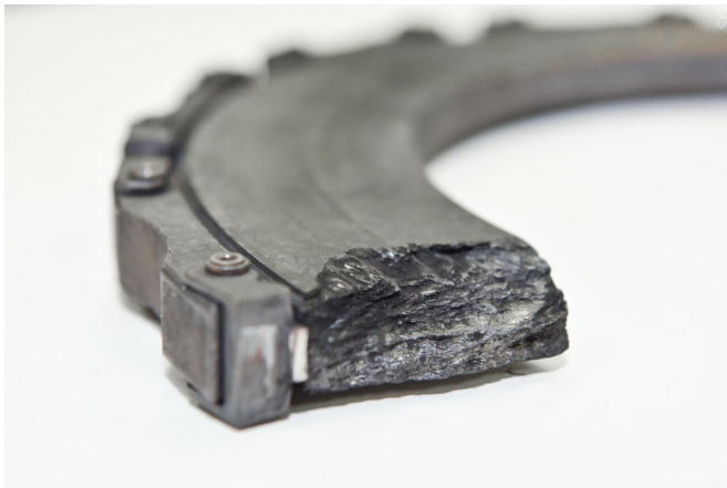
Aircraft brake disk, breakage after mechanical tests Credit: Sergey Gnuskov/NUST MISIS
