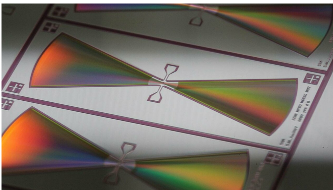
An acoustic chip is used to generate and control sound waves. Credit: Kevin Satzinger
