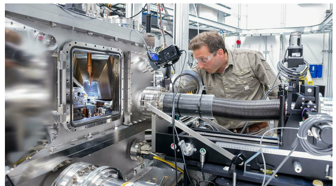
Argonne nanoscientist Martin Holt took X-ray images of the acoustic waves with the Hard X-ray Nanoprobe at the Center for Nanoscale Materials and Advanced Photon Source, both at Argonne. Credit: Argonne National Laboratory
