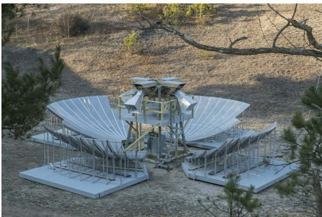
Three new dishes were added to Brookhaven's prototype radio telescope, which is stationed in an overflow basin at the Lab. Credit: US Department of Energy
