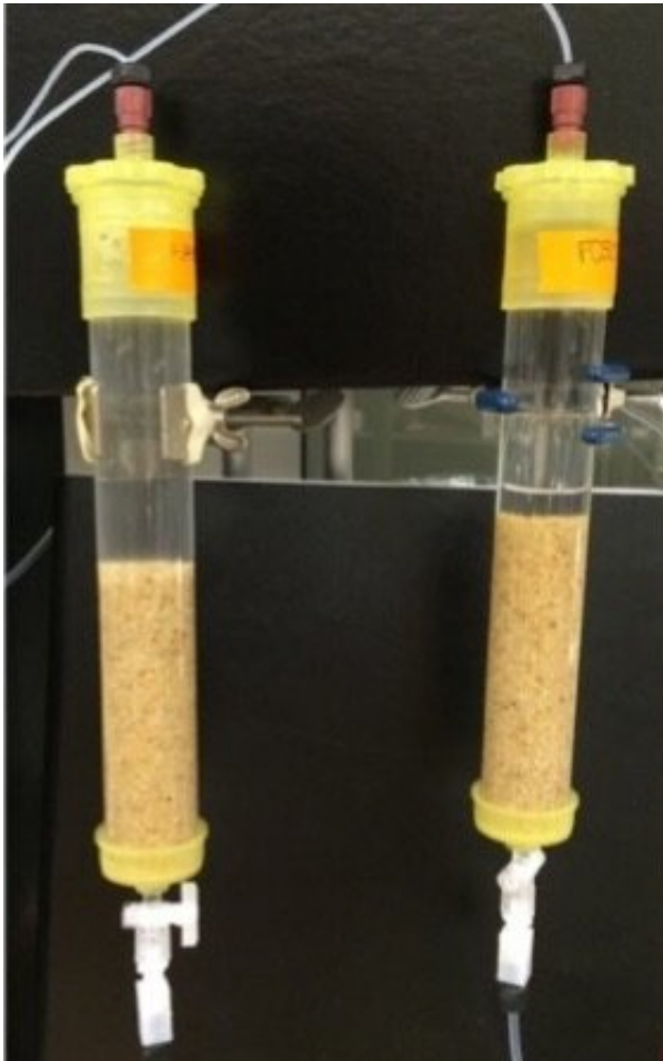
The lab-scale biofilters used during Dr. Jason Huntley's research at The University of Toledo are sand filters that contain biologically active bacteria that break down microcystin toxins. Credit: Dr. Jason Huntley, The University of Toledo
