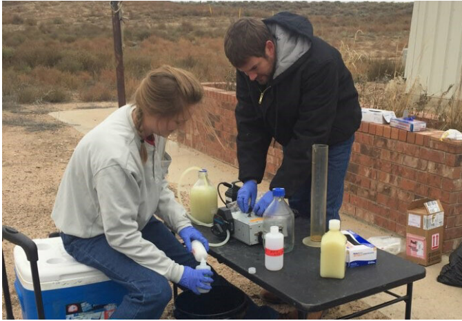
Graduate student Kaela Amundson and Michael Wilkins filtering produced hydraulic fracturing fluids in the field. Credit: Kayla Borton, CSU
