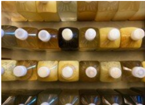
Samples of the fluids produced at a hydraulic fracturing site. Credit: Kaela Amundson, CSU
