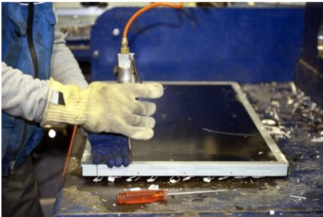
LCD screens contain small amounts of indium. From an ecological point of view, it is worth extracting the material - at least if the devices are disassembled manually. Credit: Swiss Federal Laboratories for Materials Science and Technology
