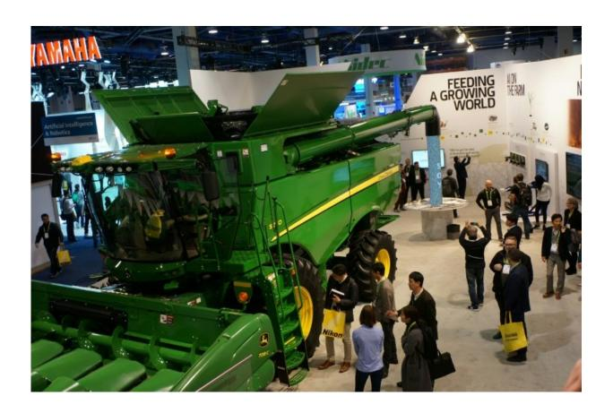
Farm equipment maker John Deere made its debut at the Consumer Electronics Show with a connected combine harvester, described as an "intelligent factory on wheels" that uses GPS, artificial intelligence and sensor technology to help improve yields
