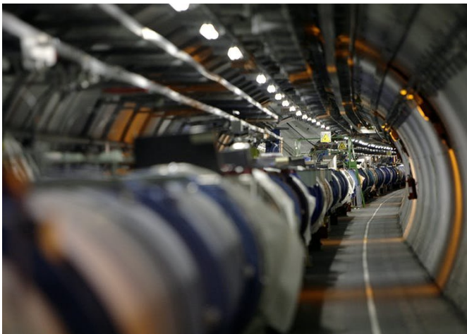
View of the Large Hadron Collider in its tunnel near Geneva, Switzerland. In the LHC two counter-rotating beams of protons are accelerated and forced to collide, generating various particles. Credit: AP Photo/KEYSTONE/Martial Trezzini
