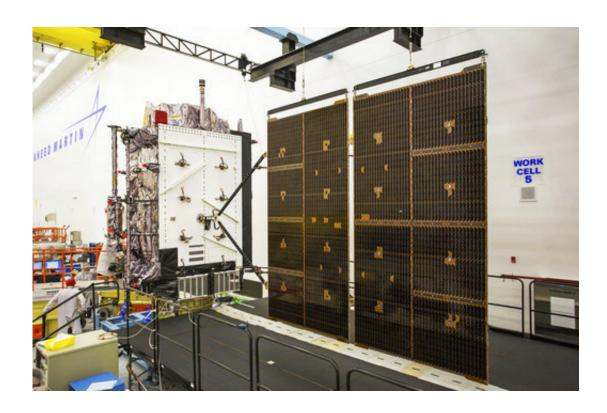
This June 23, 2017 photo provided by Lockheed Martin shows the second GPS III satellite during testing of the deployment of its solar arrays in a clean room at Lockheed Martin's complex south of Denver. The first GPS III satellite is scheduled to be launched from Cape Canaveral, Fla., on Tuesday, Dec. 18, 2018. (Pat Corkery/Lockheed Martin via AP)
