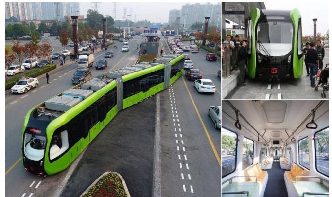
CRRC optically guided bus in Zhuzhou, China, a 3.2km system inaugurated in May 2018.
