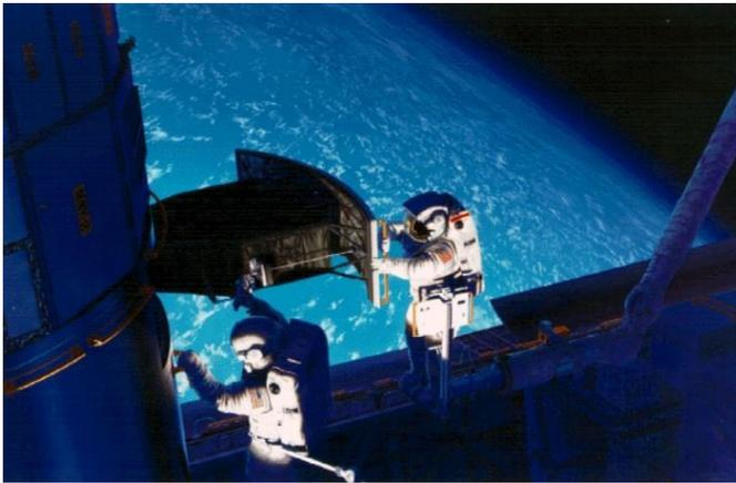
Astronauts Jeffrey Hoffman and Story Musgrave install the Wide Field and Planetary Camera 2 (WFPC2) on the Hubble Space Telescope, during SM1 in December 1993. Credit: NASA
