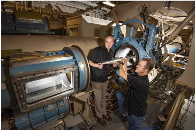
Aerospace engineer Steven Beresh, left, and technologist Russell Spillers of Sandia National Laboratories' aerosciences department place a model in the hypersonic wind tunnel's test section. Credit: Randy Montoya
