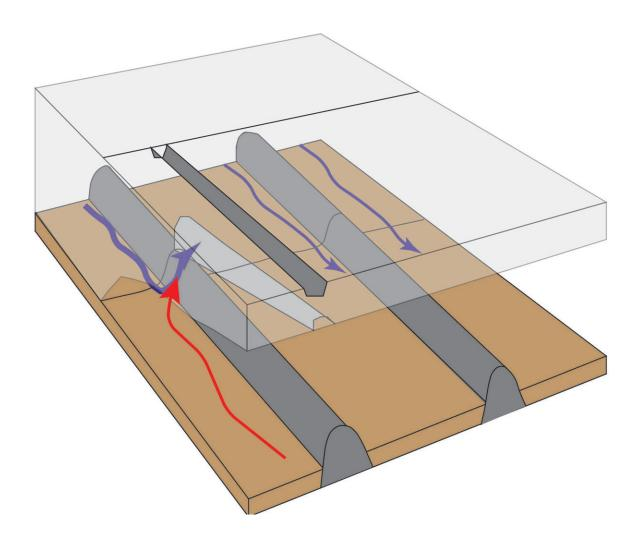
As the ice, flowing from upper-left to lower-right, encounters a hill beneath the ice (light grey shape), a cavity is created under the ice shelf. Water (red and blue arrows) feeds into the cavity, melting a channel that is reflected on the ice surface (dark grey channel). Credit: Imperial College London
