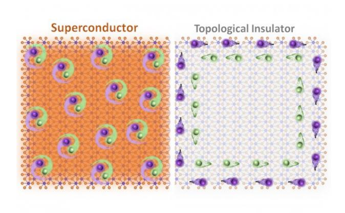
In two-dimensional tungsten ditelluride, two different states of matter — topological insulator and superconductor — can be chosen at will, MIT researchers discovered. Credit: Sanfeng Wu
