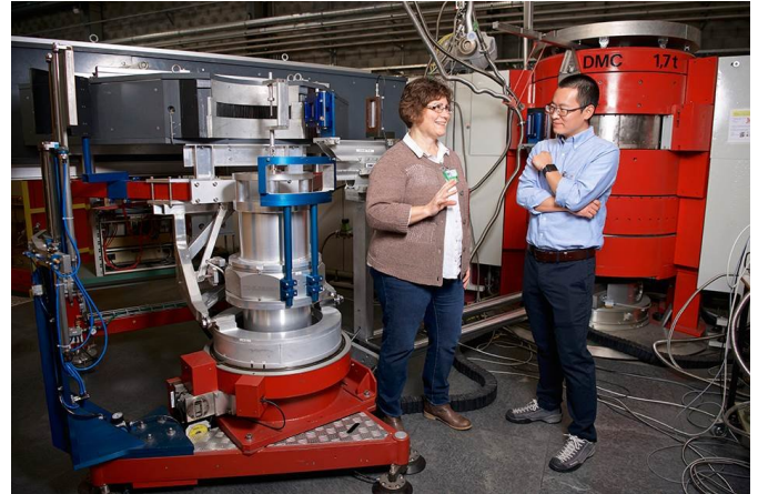
Marisa Medarde and Tian Shang at the neutron diffractometer DMC. With this device Shang found out where the atoms are located in the crystal lattice and how far apart they are from each other. Credit: Paul Scherrer Institute/Markus Fischer
